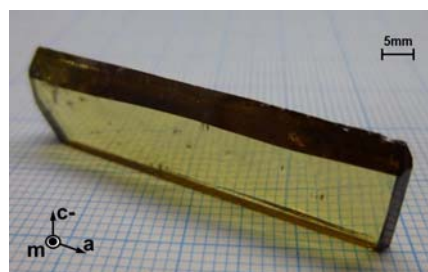
Fig.2 m -plane crystal, radius of curvature: 1460m
